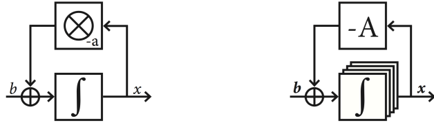
Figure 10.2: How feedback in an analog computer circuit can be used to implement scalar division (left) and solving for the solution vector of a linear algebra problem (right).
